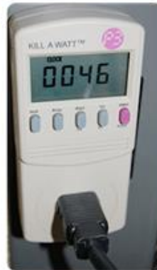
The Kill A Watt™ displays a bevy of information such as kWhs used, plug-in time, voltage, current, watts and more.
